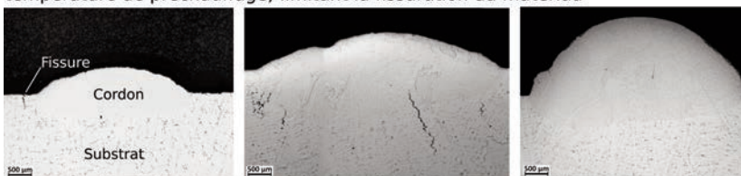
Fissuration en surface
