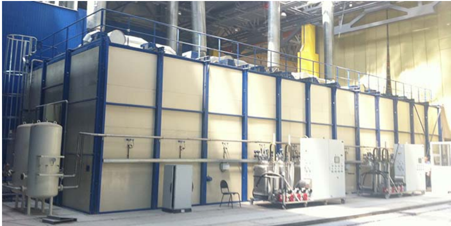
Figure 1. 20 m long Infusion Oven
