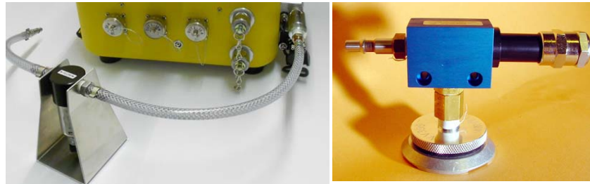
Left : Filter on purging air circuit; right: Venturi vacuum pump mounted on its bag valve
