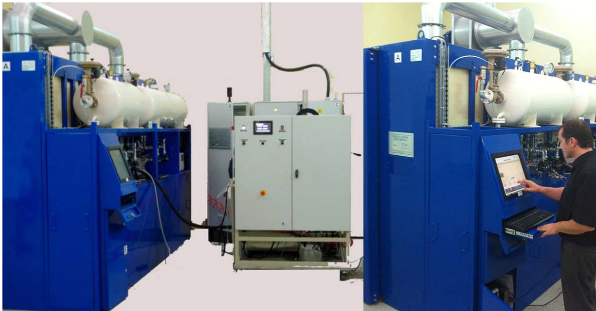
Figure 2. OVEN with Infusion machine ; our coordinated control software ANICURE
